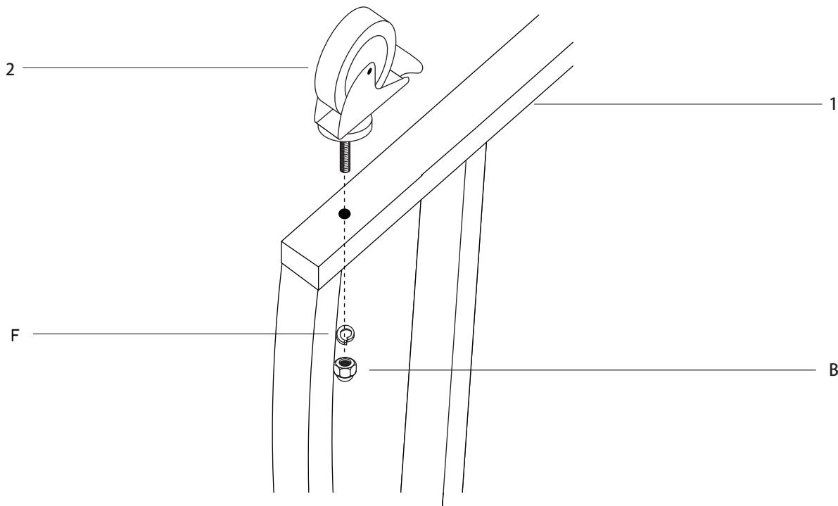
**STEP 1** - Attach the four pre-threaded castor wheels (2 & 3) to each of the four brackets (1) by pushing them through the hole. Using an adjustable spanner secure each castor wheel with 1x nut (B).
