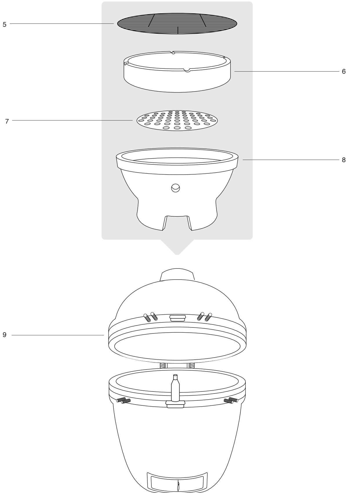
**STEP 8** - When the grill is securely placed on the cart add the firebox (8), charcoal plate (7), upper ring (6) and cooking grill (5) inside of the Kamado Grill as displayed in the assembly diagram.
