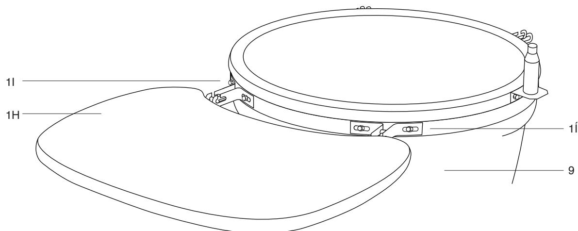
**STEP 14 -** Insert the 2x table hinge into each of the table brackets (14 & 15).
