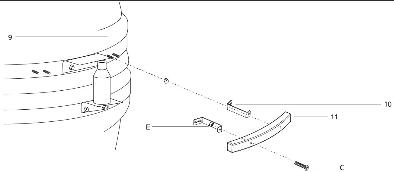
**STEP 10 -** To attach the handle (10) to the lid of the Kamado Grill (9) start by attaching 2x handle brackets (11) using the 2x pre-attached bolts and dome headed nuts. Attach the handle (11) to the brackets (10) using 2x bolts (C) and nuts (E).
