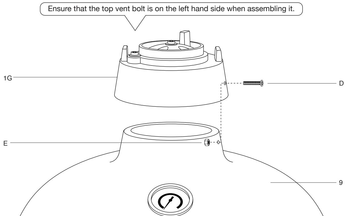
**STEP 11 -** To attach the top vent (12) to the Kamado Grill (9) place it on top and align both the bolt holes. Secure using 2x bolts (D) and nuts (E). Ensure that the top vent bolt is on the left hand side when assembling it.
