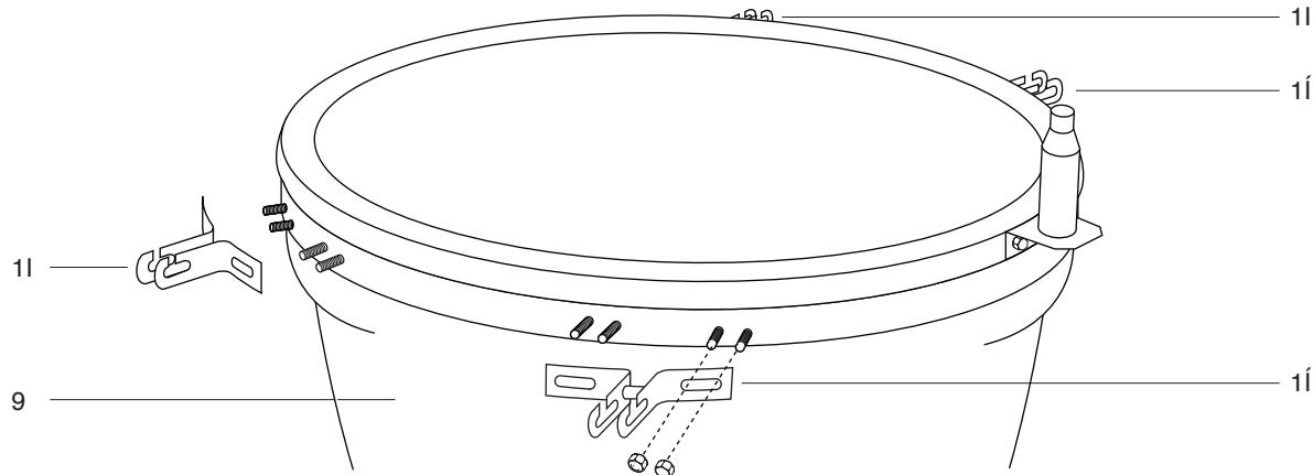
**STEP 12 –** Attach the 2x table brackets (14) to the Kamado Grill (9) using the 4x pre-attached bolts and dome headed nuts per bracket. Please note the position shown in the above diagram
